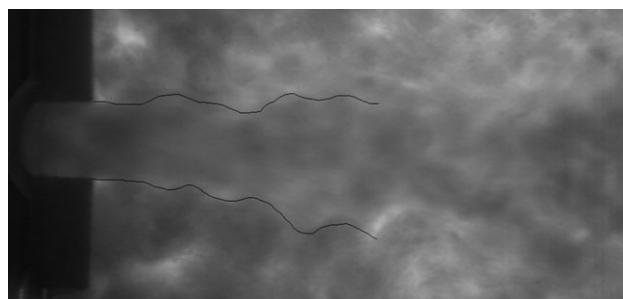
Figure 2. High-speed camera picture of the jet at a concentration of 1.8% and an average inlet velocity of 1.5 m/s at x = 0 .
